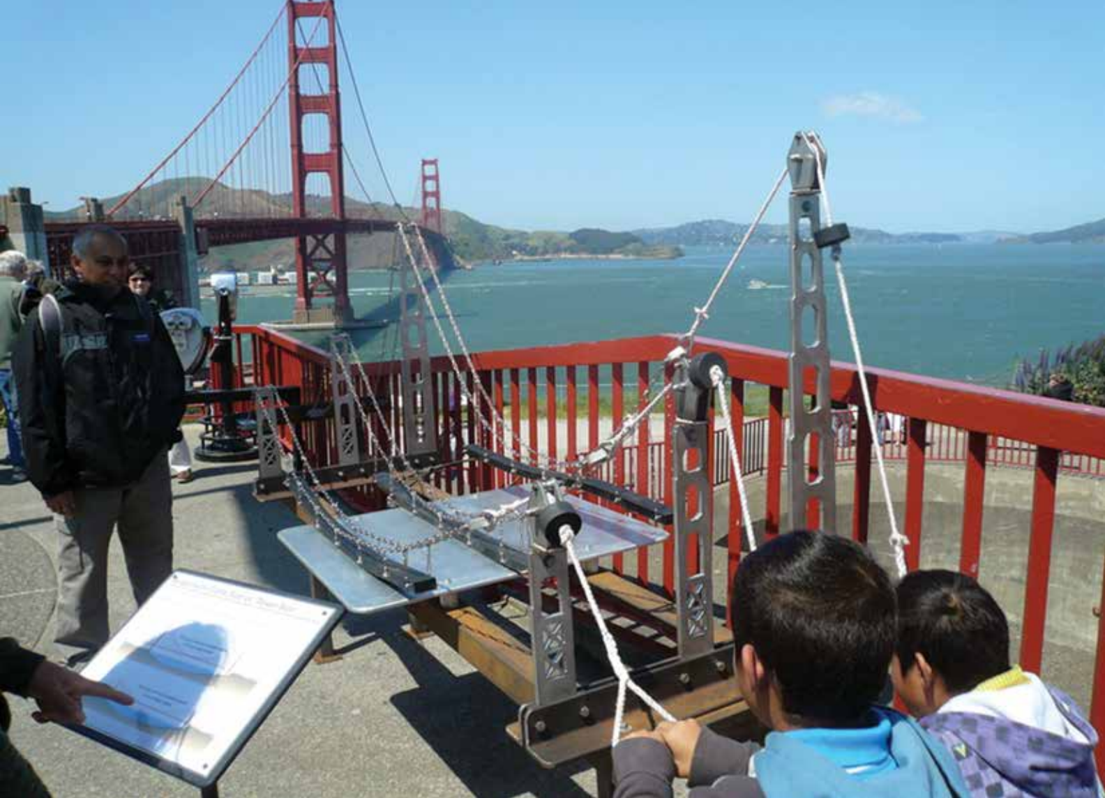
This exhibit shows three possible heights for the towers of the Golden Gate Bridge. The greater the distance from top of the towers down to the bottom of the sag of the cables, the more efficiently the cables can lift the weight of the deck. The trade-off is that the cost and difficulty of building taller towers would have outweighed that cost savings. Exhibit design by David Fleming, the Exploratorium. Photo courtesy Golden Gate Bridge Highway and Transportation District
